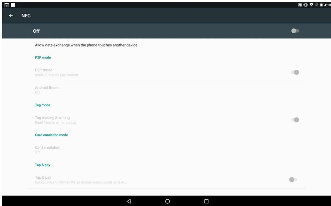
Open the Setting,find the More...,select the NFC , the antenna on the back,put the tag near the antenna, the device will make a sound.
